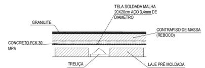
07 DETALHE LAJE PRÉ MOLDADA
